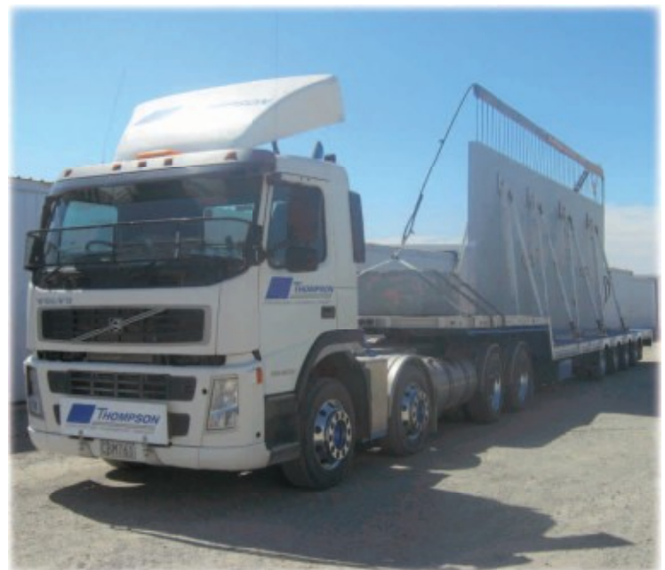
Panel ready to be transported to site
